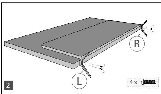
(fig.2) Secure the stand/feet to the underside of the TV set using the 4 screws provided.
