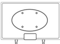
1) Remove the four screws located at the back of the TV set.
